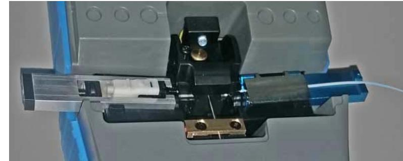
After splicing, the connector fits in the oven to heat-shrink a protective sleeve over the fiber.
